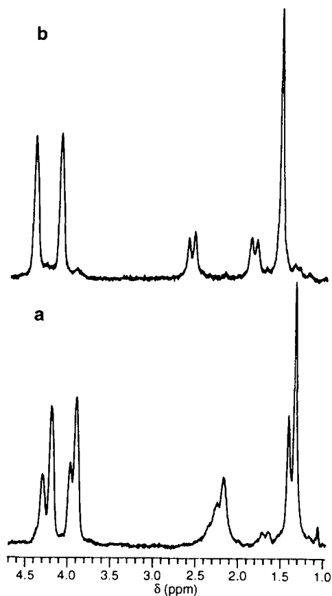
Figure 4 ^1\text{H} n.m.r. spectra in the aliphatic proton region of (a) radical and (b) anionic poly(MEAB), in toluene- d_6 at 100 C
